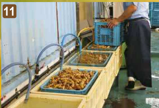
The crates of Ukon are soaked and sanitized in larger containers of running Strong Acidic (pH2.5) Water for 2-5 minutes.
