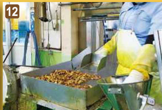
The Ukon is washed through a hot shower as it is loaded into the next room, where a worker scoops them into a slicing machine. The thinly (1mm) sliced Ukon is gathered in a larger, wide container as it shoots out of the slicing machine.
