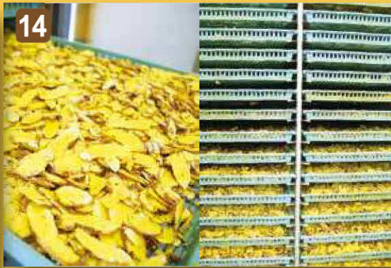
The Ukon trays are slid into a heat-dryer for about 7 hours in 72°C (161.6°F)
