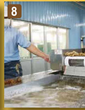
Factory workers check for leaves, grass, stones, etc., and break the Ukon into smaller pieces before they are cleaned in a small pool of jet water.
